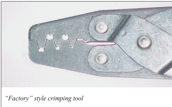
For small wires, snip off a portion of the crimp - it will make a neater crimp this way.
