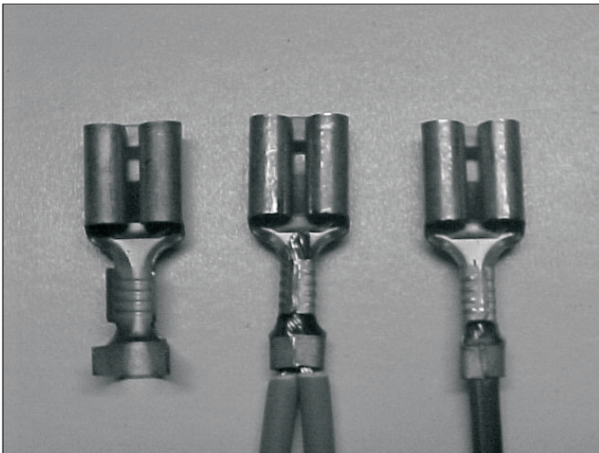
Crimp the wiring/terminals using a pair of pliers. The lower crimp should be over the insulation for a one-wire crimp, and over the bare wires only for a two-wire crimp.
