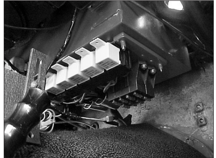
Power Block as installed in a TR3. In this car, the best location for the block was under the battery box, behind the dash, but a suitable location can be found in any car.
